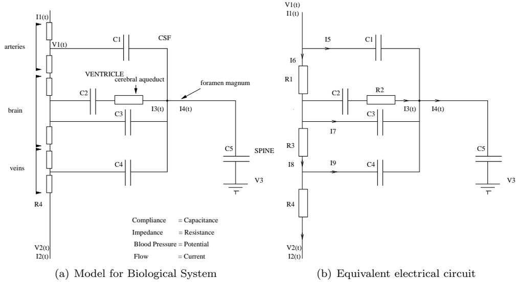
Figure 3: Electrical Circuits for the Simplified Biological Model.
