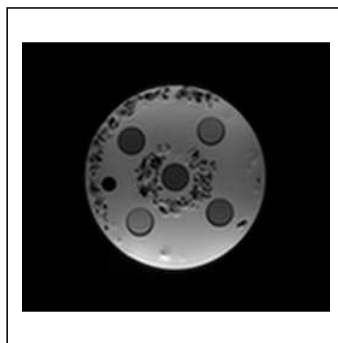
Figure 7: A sample image slice ( b = 100 ) from the new diffusion data where a marker has been added to determine the orientation of the phantom.
