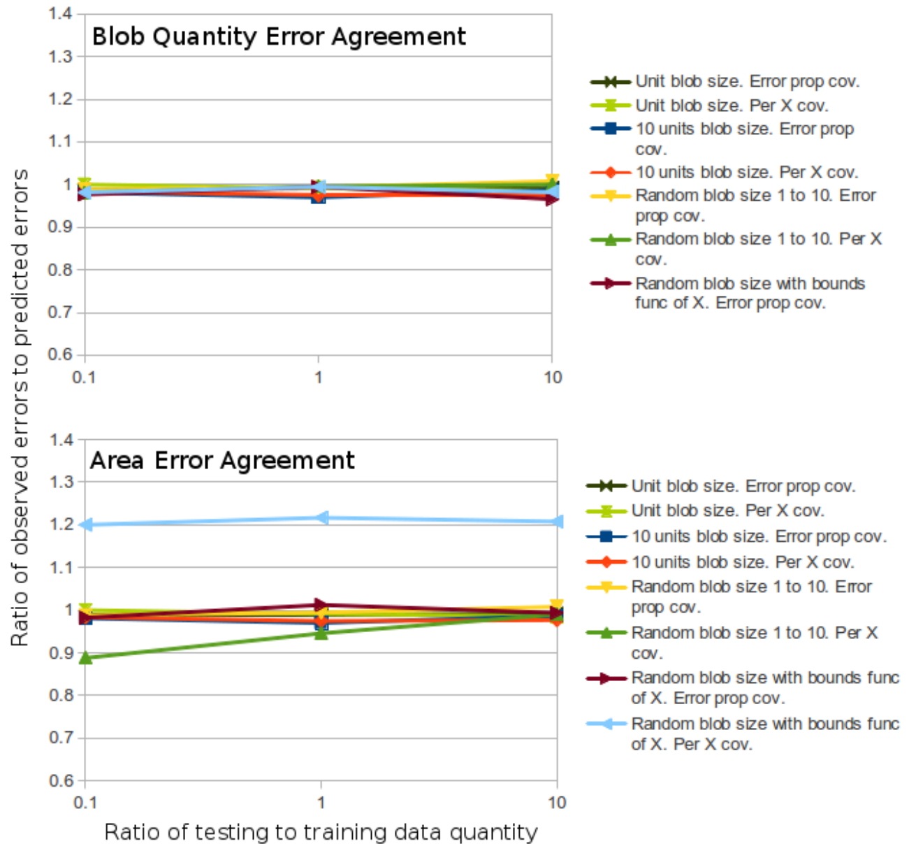
Figure 2: Comparison of error estimation methods using fixed and random blob sizes. The error propagation method produces consistent predictions of error (ratio of observed to predicted errors of unity) over all tests and relative quantities of testing to training data. The per-X covariance scaling method fails to produce consistent error estimates on areas when the random blob sizes are selected with bounds which are a function of X.
