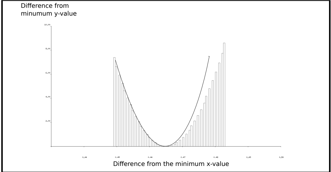
Figure 2: Plot of the cost function. The skew of the quadratic function is typical of a cost function in heteroscedastic space. The minimum of the quadratic function represents the converged value of the cost function.
